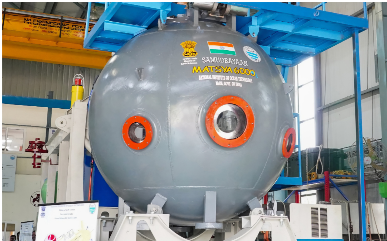
Matsya 6000, Human Support and Safety System, built by Unique Group.
