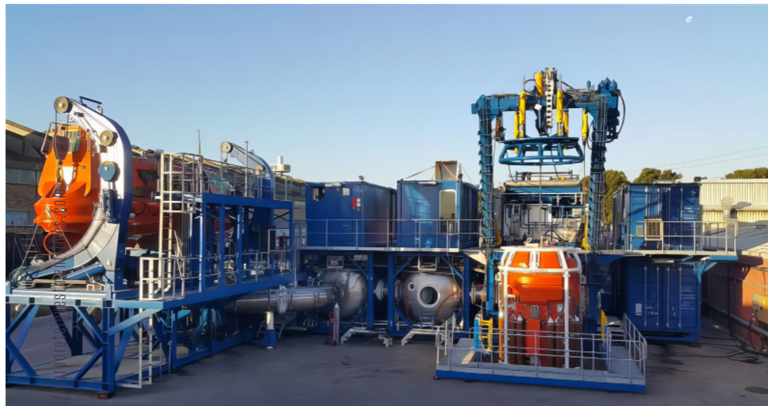
A DNV classed 12 man 300 msw rated customised saturation diving system
