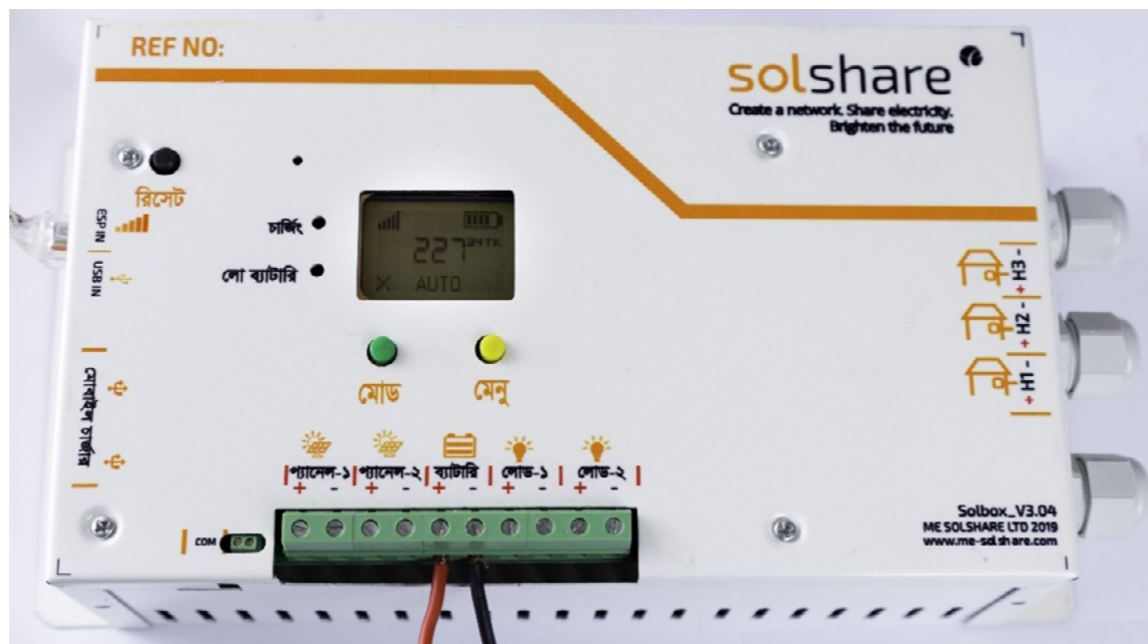
SOLshare's SOLbox: The SOLbox NG, a smart bi-directional meter which acts as the point of interconnection within the P2P solar microgrids.
