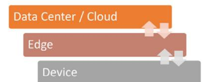
concept of Metaverse applications that demand real-time/predictable latency (industrial automation, transportation, networks of sensors and actuators). Edge Computing paradigm is well positioned for real time Big Data and real time analytics, it supports densely distributed data collection points, hence adding a fourth axis to the often-mentioned Big Data dimensions (volume, variety, and velocity).
